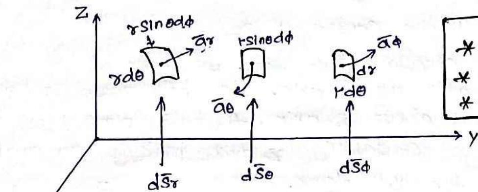
$$\begin{aligned} * d\bar{S}_r &= r^2 \sin\theta d\phi \\ * d\bar{S}_\theta &= r \sin\theta dr d\phi \\ * d\bar{S}_\phi &= r dr d\theta \end{aligned}$$
