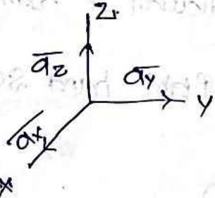
$$* \bar{a}_x \times \bar{a}_y = |\bar{a}_x| |\bar{a}_y| \sin \theta \cdot \bar{a}_N \\ = 1 \times 1 \times 1 \bar{a}_N$$
