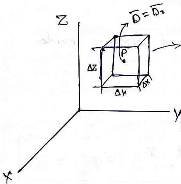
Rectangular box as closed differential Gaussian surface
