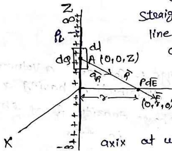
Consider an infinitely long straight line carrying uniform line charge having density  $\rho_L$ . Let this line lies along z-axis from  $-\infty$  to  $\infty$  and hence called infinite line charge.
